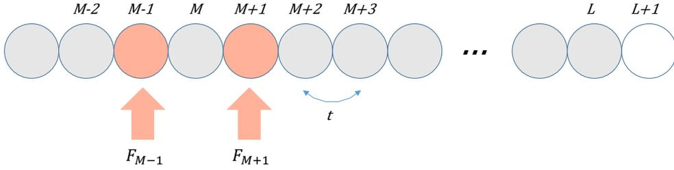
Fig. S2. Schematic representation of a one-dimensional lattice with two pump drives at sites  $M-1$  and  $M+1$ . The site  $L+1$  is out of the lattice.
