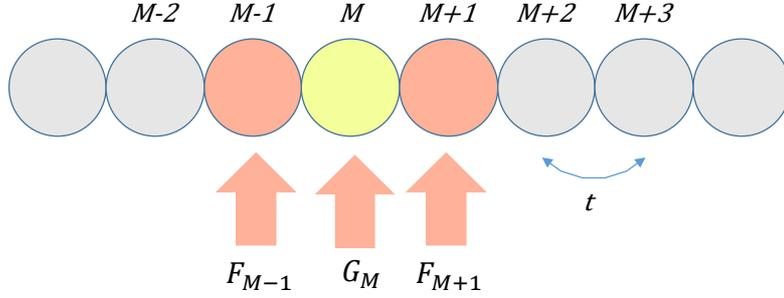
Fig. S4. Schematic representation of a one-dimensional lattice with two pump drives at sites  $M - 1$  and  $M + 1$  and an additional drive at site  $M$ .
